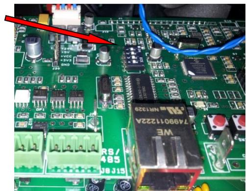
Figure 10 - Configuration dip-switches
