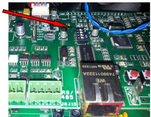
Figure 10 - Configuration dip-switches
