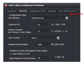
Figure 3 - Settings for n. 1 Pylontech US2000B / Extra 2000 battery
