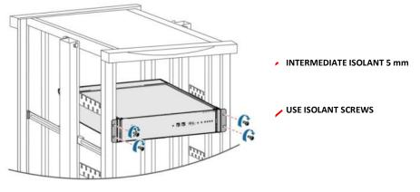
Figure 1 - Pylontech battery fixing
